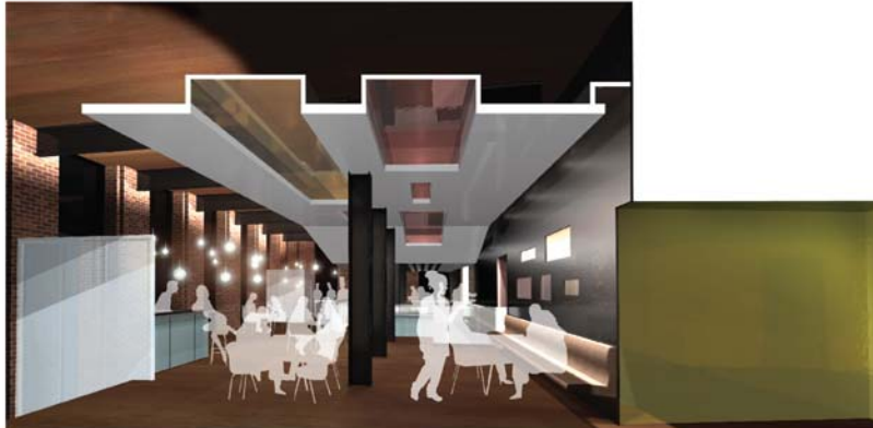
View of the Dining Room and Acoustical Ceiling Treatment
